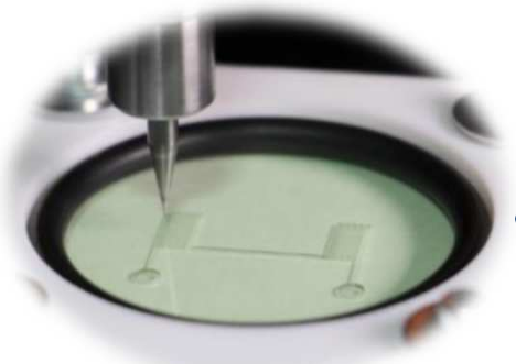
10 \mu\text{m} \varnothing tools / optical finish
