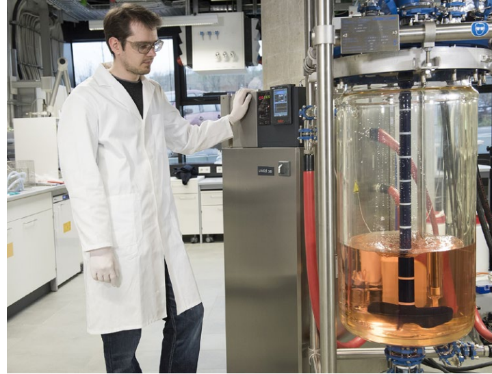
The Ruhr reactor for particle synthesis with a 100-liter capacity
