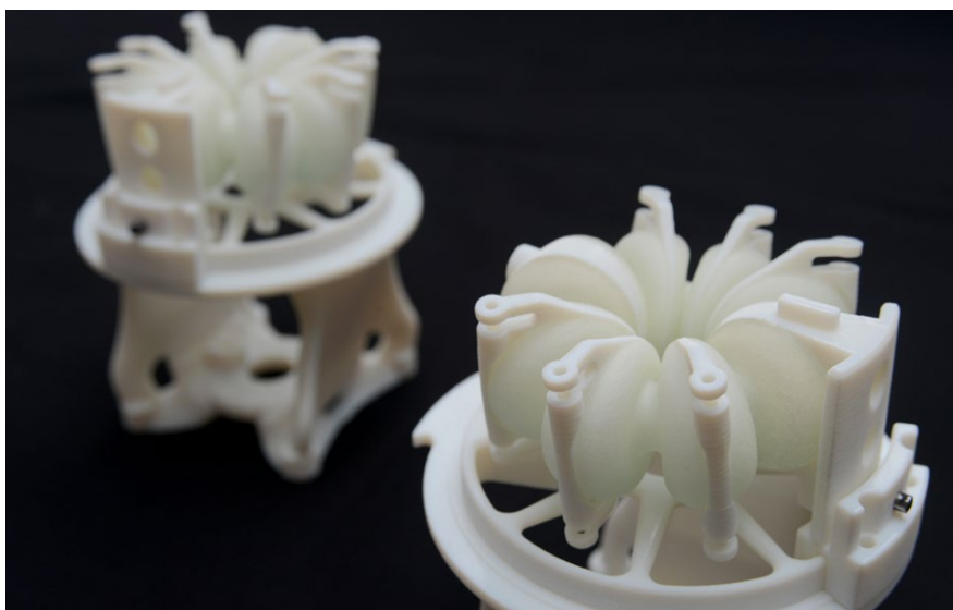
Maximum functional integration permitted the pneumatic Festo robot actuator to be printed in one step.
