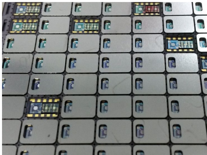
Batch of sensor pre-concentrator systems partially covered by a precisely positioned gas inlet
