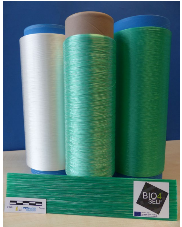
Self-reinforced fiber composite plastic (eFVK) made of PLA and PLA fibers
