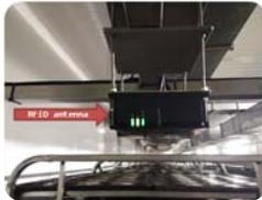
RFID antenna reading RFID tag
