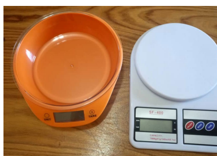
a. Electronic balance with precision of 0.5 grams
