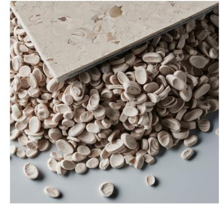
The calcium carbonate to be produced by Ragn-Sells could be used as mineral fillers for Tarkett vinyl flooring. Several hundred thousand tons of mineral fillers are used by Tarkett every year. Photo credits: Philip Gatward
