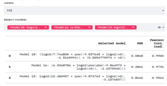
The maximum hydrogen concentration is estimated by models for the gasification temperature 900 - 1,000 ° C
