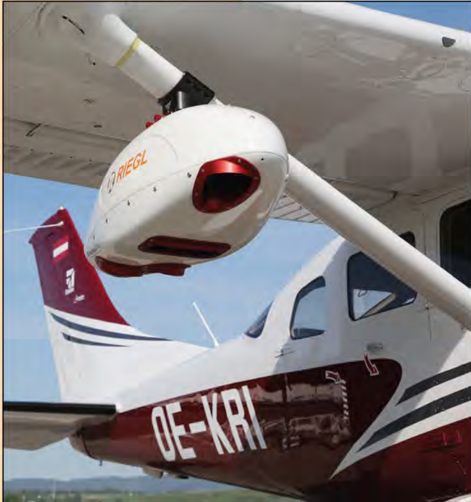
RIEGL's Cessna T206H test plane equipped with VQX-1 wing pod
